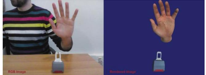
*Tracking object and hand poses using a 3D camera. The 6 DOF position and orientation of the object is tracked while 42 DOFs of the hand are estimated.*
